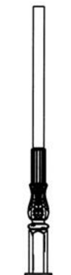
Ø40mm TOP 80 x 80mm BASE CAST POST
