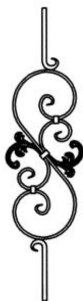
EIW 141 □12-16 / Ø14mm SCROLLS : 16 x 8 / LEAF CAST 580 H x 215 W HEB / PL
